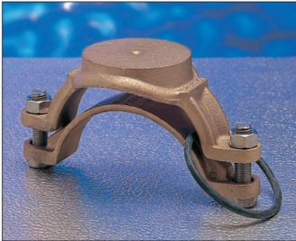
into the boss of the strap and tapings from 1/2" to 2" can be made into most flat boss straps. Alternatively the strap can be pre-drilled and tapped and fitted with a ferrule prior to delivery for use on asbestos cement and PVC mains. The wall of the pipe is then simply drilled using under pressure drilling equipment.
