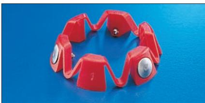
The grip ring's flexibility allows it to be compressed inwards when pushed down the tapered mouth of the fitting. This enables Grippa to join a wide range of pipe types and sizes. The patented grip ring has two sets of gripping teeth. Firstly, six sets of moulded plastic teeth to provide a uniform, secure grip onto the softer lead pipes. For harder copper and galvanised iron there is a secondary set of three stainless steel studs which grip securely into the surface of the pipe.
