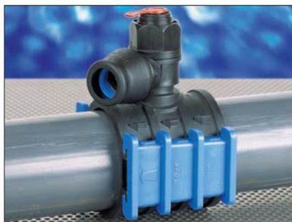
*The Talbot all Plastic Self Tapping Ferrule Strap is a design that combines tried and tested technology with revolutionary design concepts. Suitable for use on PVC or PE pipe, the Talbot Plastic Self Tapping Ferrule Strap is lightweight and can be used in any situation in place of a welded or traditional gunmetal strap. When used in conjunction with the Talbot Grippa it allows new service provision to properties with existing lead, galvanised iron or copper service supply pipes*
