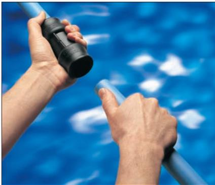
*Talbot Pushfit fittings are quick and easy to use, with no nuts to lose or leave undone. Simply push the pipe into the fitting. The grip and seal on the pipe increases with pressure and tensile load so that the pipe will burst or neck before the fitting will fail. The Talbot Grippa enables new PE distribution networks created using the Talbot Pushfit connection to be connected to existing service pipe of lead, galvanised iron or copper.*
